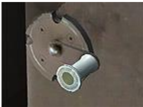
Rudder pedals adjustment crank (2)
