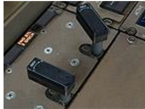
Engine fuel shutoff handles (3)
