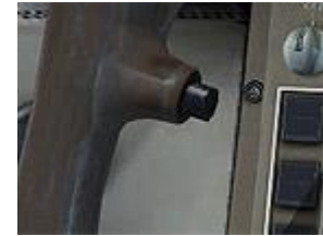
Control wheel autopilot switch
