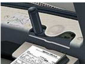
Pilots' windows handles and mechanism (2)
