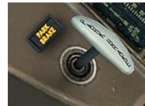
Parking brakes control lever
