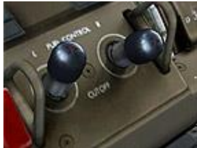
Engine fuel cutoff handles (2)
